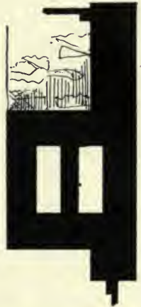
• CHIMNEY AT ATTIC •
